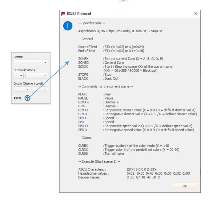
Connect the RS232 transmitter to the interface RS232 (Tx, Rx and GND pins) and send the dedicated ASCII commands lines that you need.
